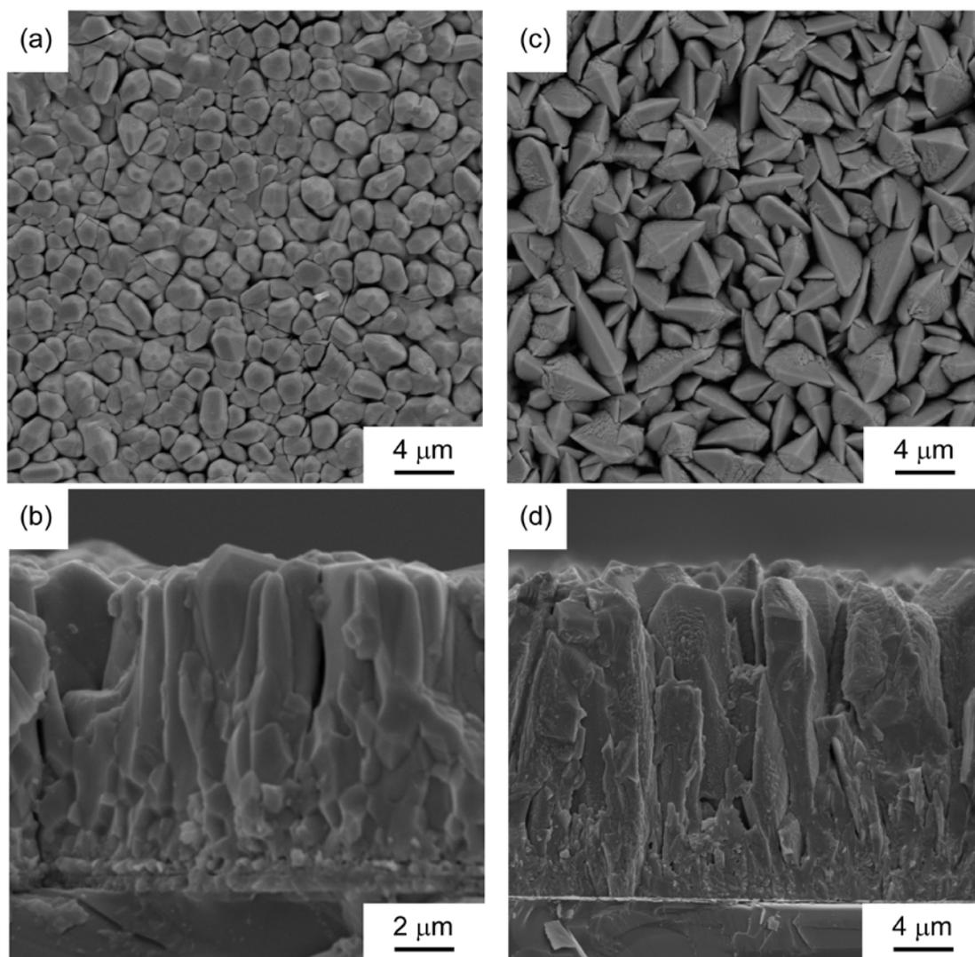
**Figure 2.** Surface (a, c) and cross-sectional (b, d) SEM images of the  $\text{Ba}_2\text{TiO}_4$  thick film prepared at 894 K (a, b) and  $\text{Ba}_4\text{Ti}_{13}\text{O}_{30}$  thick film at 997 K (c, d).
