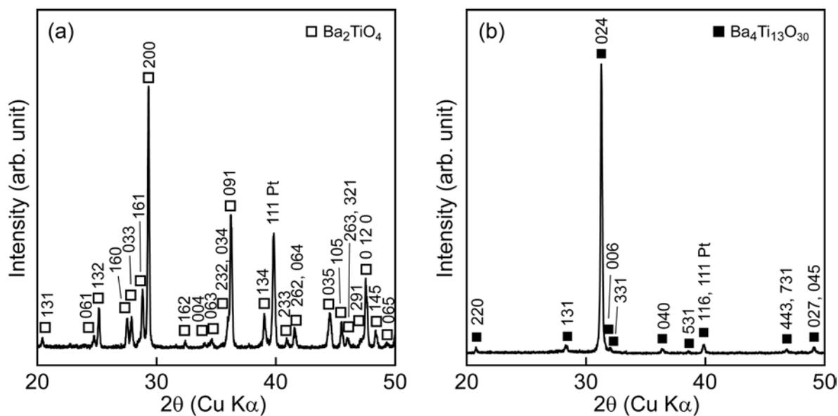
**Figure 1.** XRD patterns of the  $\text{Ba}_2\text{TiO}_4$  thick film prepared at 894 K (a) and  $\text{Ba}_4\text{Ti}_{13}\text{O}_{30}$  thick film at 997 K (b).
