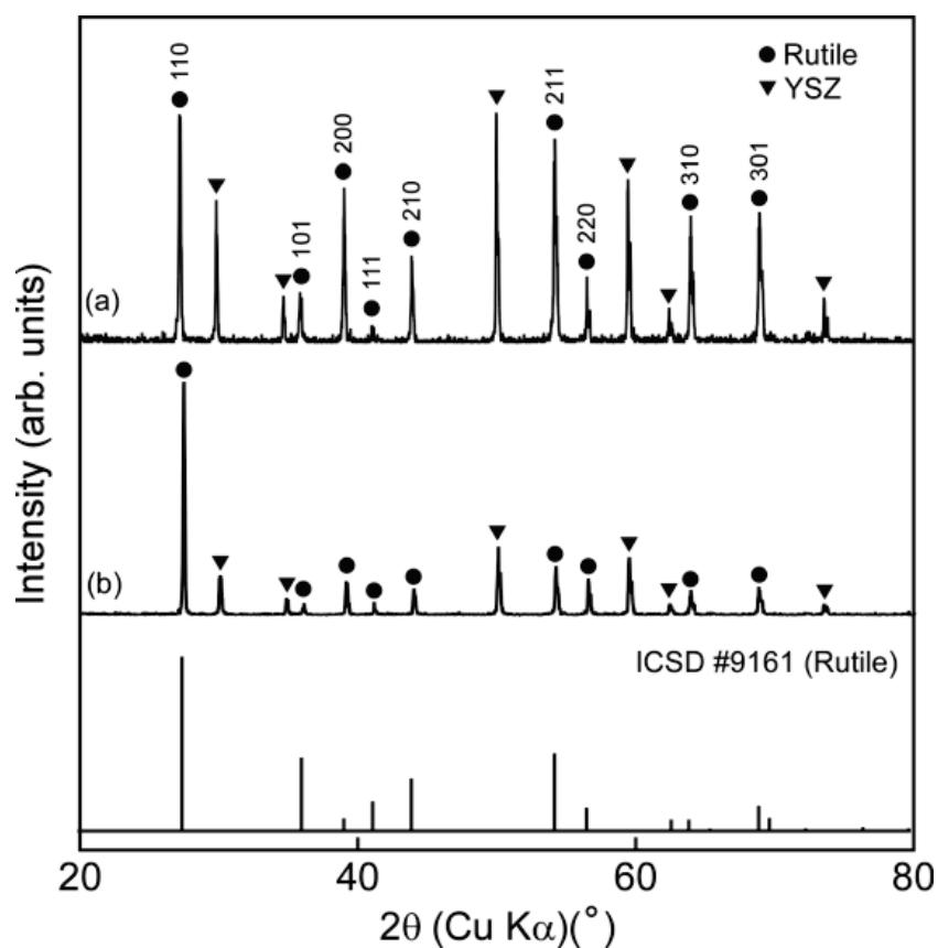
**Figure 2** XRD patterns of  $\text{TiO}_2$  films prepared using  $\text{CO}_2$  laser at  $P_{\text{tot}} = 0.4 \text{ kPa}$  and various  $T_{\text{dep}}$ : 1020 K (a) and 1078 K (b).
