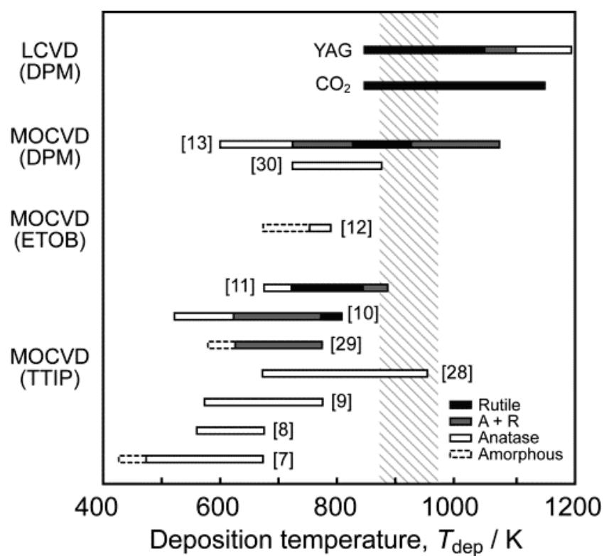
**Figure 14** Anatase and rutile formation in TiO<sub>2</sub> films prepared by MOCVD and present LCVD. TTIP: titanium tetraisopropoxide, ETOB: titanium ethylacetoacetate, DPM: titanium dipivaloylmethanate. Hatched region indicate the temperatures for anatase-to-rutile transition [4].
