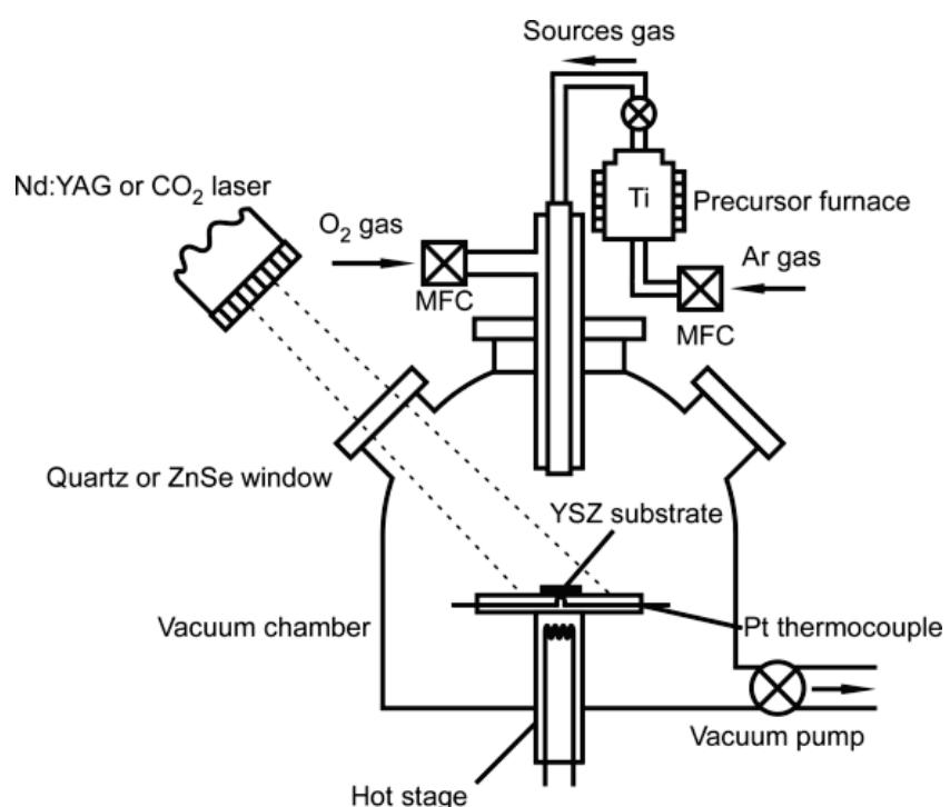
**Figure 1** A schematic of laser CVD equipment.
