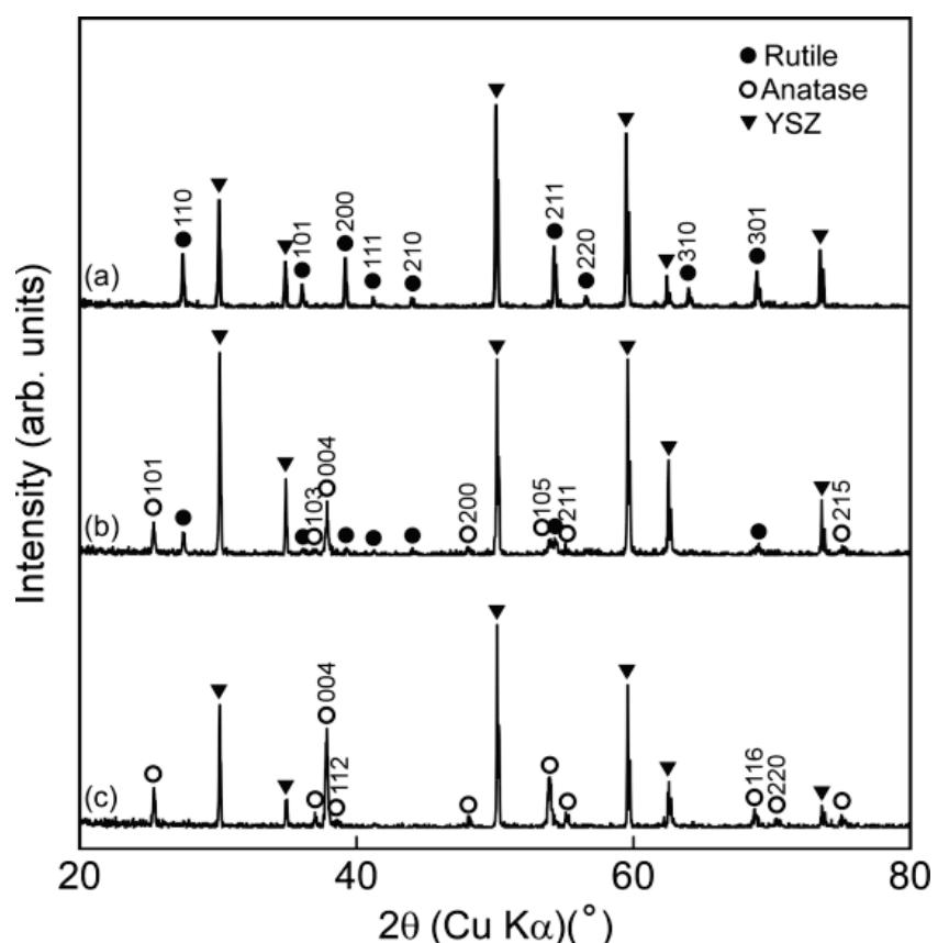
**Figure 8** XRD patterns of  $\text{TiO}_2$  films prepared using Nd:YAG laser at  $P_{\text{tot}} = 0.6$  kPa and various  $T_{\text{dep}}$ : 1047 K (a), 1072 K (b) and 1142 K (c).
