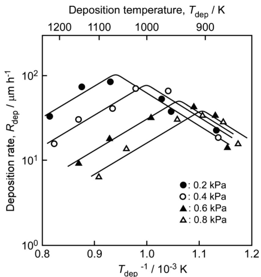
**Figure 7** Effect of  $T_{\text{dep}}$  and  $P_{\text{tot}}$  on  $R_{\text{dep}}$  of  $\text{TiO}_2$  films prepared using  $\text{CO}_2$  laser.
