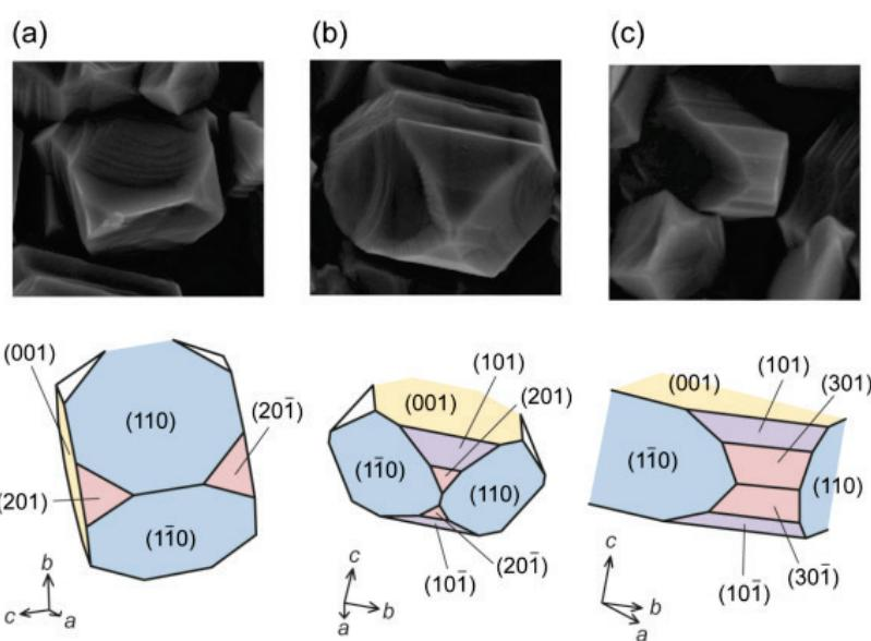
**Figure 5** Pyramidal-shaped grains in the rutile  $\text{TiO}_2$  films prepared at  $P_{\text{tot}} = 0.2 \text{ kPa}$  and  $T_{\text{dep}} = 1078 \text{ K}$  and their crystal shapes.
