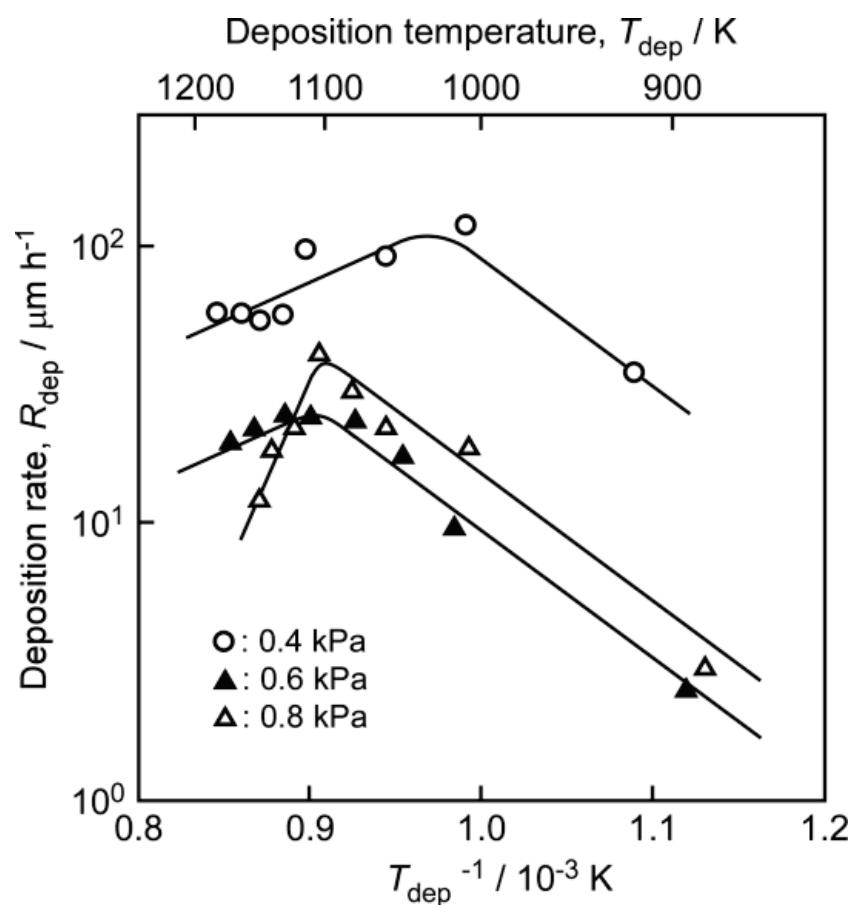
**Figure 13** Effect of  $T_{\text{dep}}$  and  $P_{\text{tot}}$  on  $R_{\text{dep}}$  of  $\text{TiO}_2$  films prepared using Nd:YAG laser.
