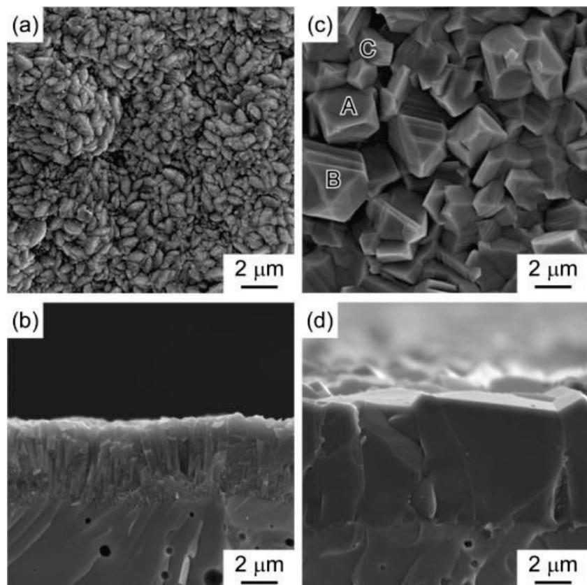
**Figure 4** Surface (a, c) and cross-sectional (b, d) SEM images of TiO<sub>2</sub> films prepared using CO<sub>2</sub> laser at various  $P_{\text{tot}}$  and  $T_{\text{dep}}$ : 0.8 kPa and 853 K (a, b), 0.2 kPa and 1078 K (c, d).
