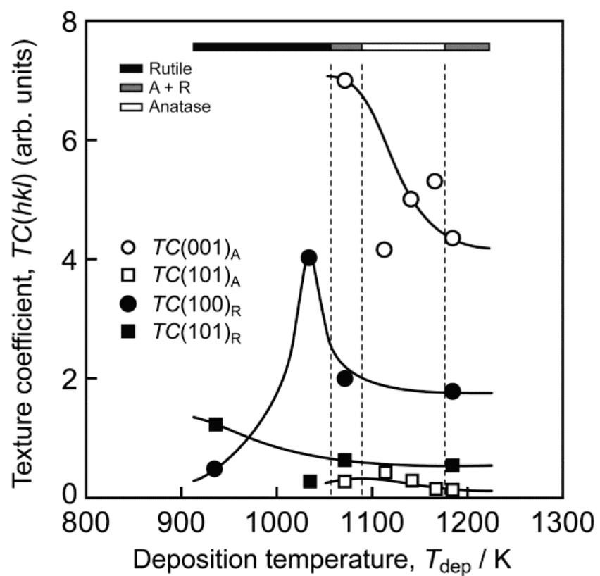
**Figure 9** Effect of  $T_{dep}$  on  $TC(hkl)$  of  $\text{TiO}_2$  films prepared using Nd:YAG laser at  $P_{tot} = 0.6 \text{ kPa}$ .
