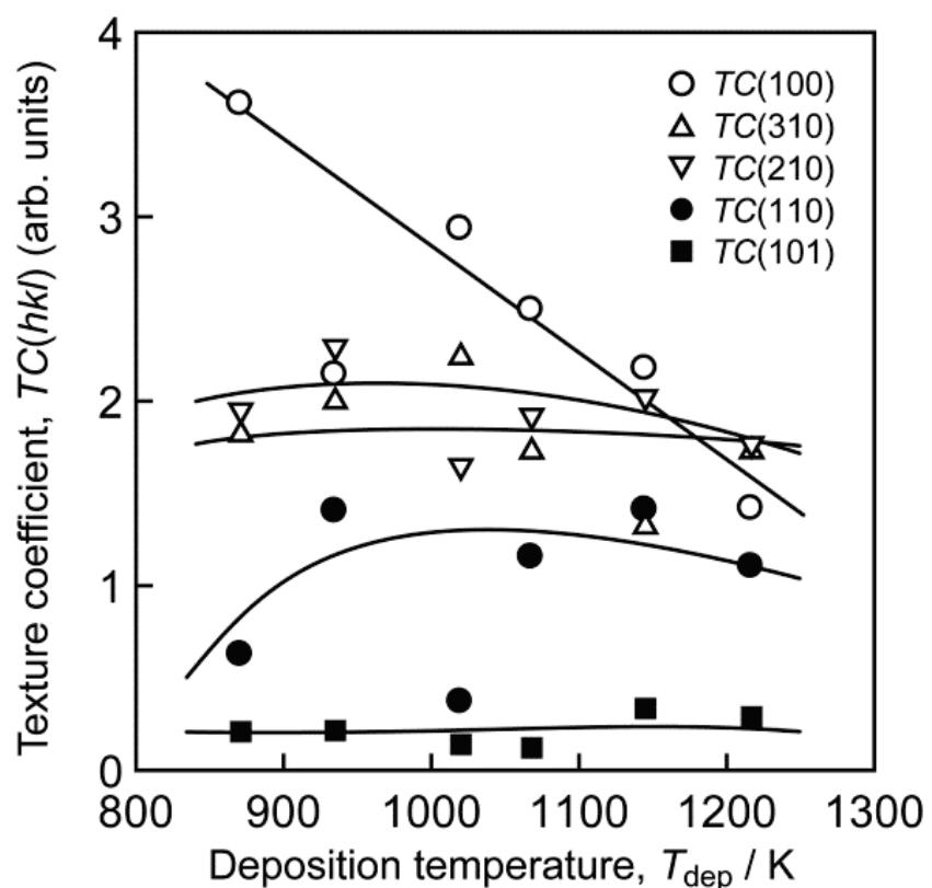
**Figure 3** Effect of  $T_{dep}$  on  $TC(hkl)$  of  $\text{TiO}_2$  films prepared using Nd:YAG laser at  $P_{tot} = 0.6 \text{ kPa}$ .
