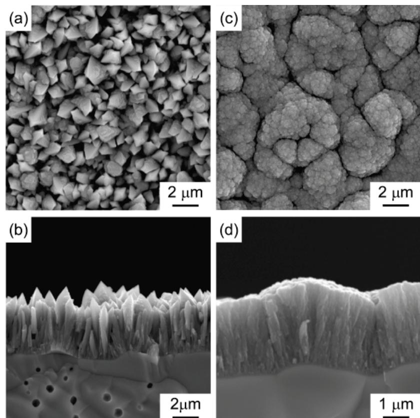
**Figure 10** Surface and cross-sectional SEM images of TiO<sub>2</sub> films prepared by Nd:YAG laser at  $P_{\text{to}\ t} = 0.6 \text{ kPa}$  and different  $T_{\text{dep}}$ : 1035 K (a, b) and 1142 K (c, d).
