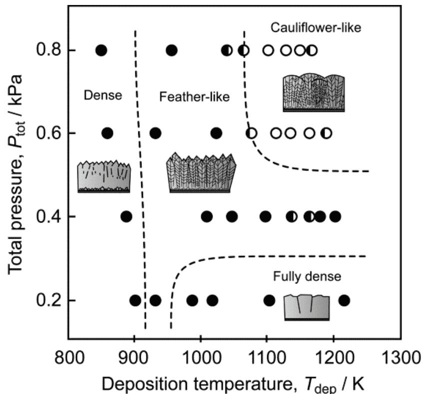
**Figure 12** Effect of  $T_{\text{dep}}$  and  $P_{\text{tot}}$  on the phase and microstructure of  $\text{TiO}_2$  films prepared by Nd:YAG laser. Filled, half-filled and open circles indicate rutile, mixture and anatase formation, respectively.
