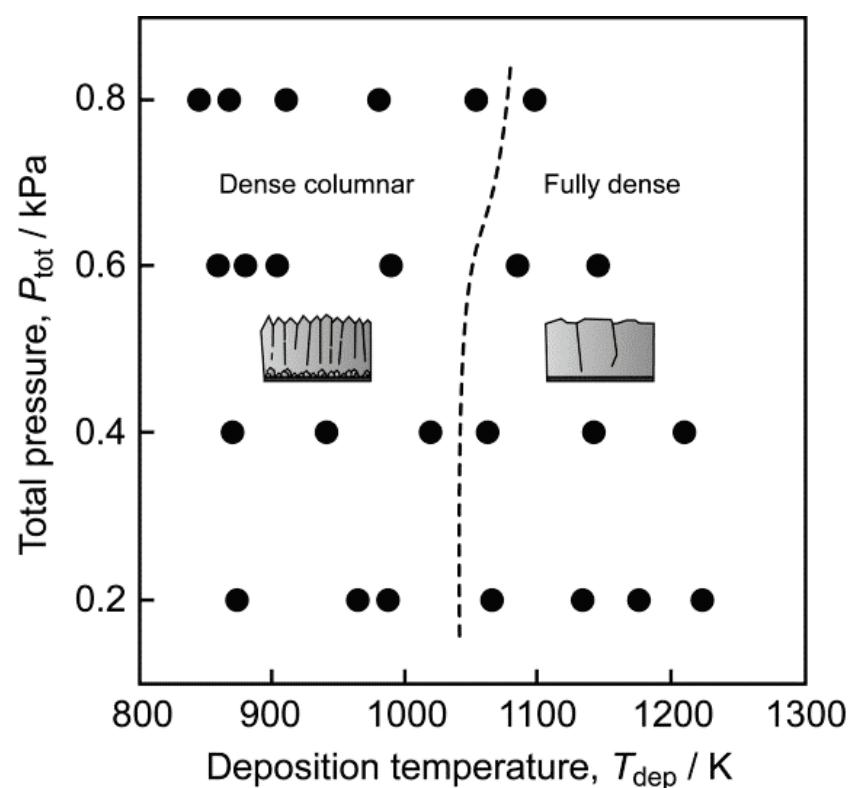
**Figure 6** Effect of  $T_{\text{dep}}$  and  $P_{\text{tot}}$  on the phase and microstructure of  $\text{TiO}_2$  films prepared using  $\text{CO}_2$  laser. Filled circles indicate the rutile formation.
